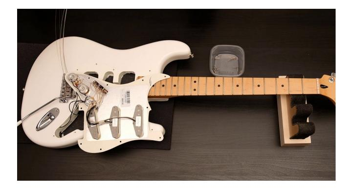
**3.** Unsolder or cut the wires coming from the output jack close to the potentiometer.
